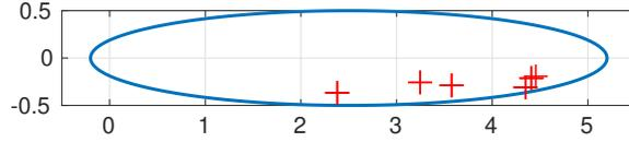
Figure 3: Transmission eigenvalue problem for the unit cube: Computed eigenvalues of the transmission eigenvalue problem by the contour integral method for  $h = 0.177$ .
